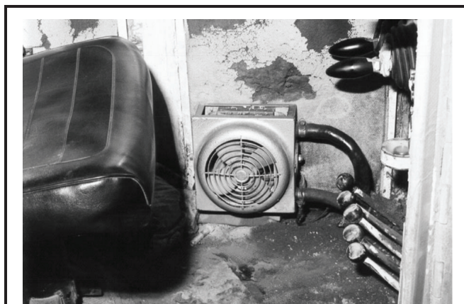
FIGURE 2. Floor heater inside enclosed cab
