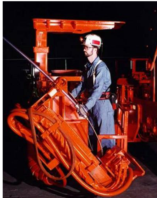
Figure 9. A hydraulic resin inserter better enables the roof bolter operator to reach the rib while remaining in the platform.
