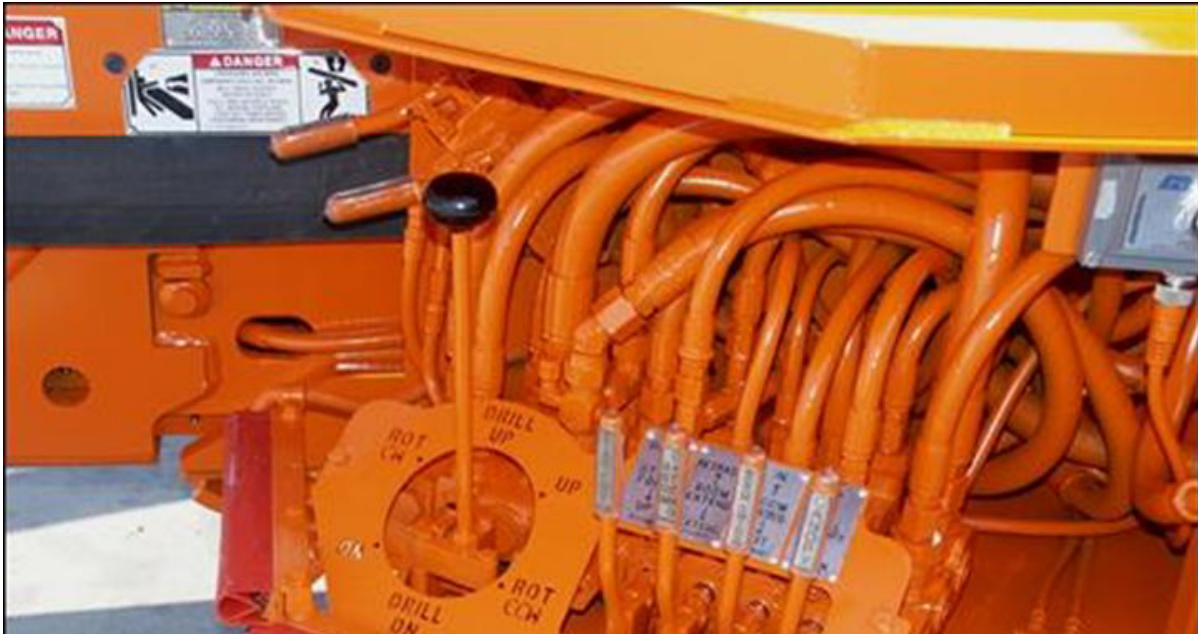
Figure 10. This new, single-lever joystick handle function is regarded as the preferred method for operating a roof bolter.
