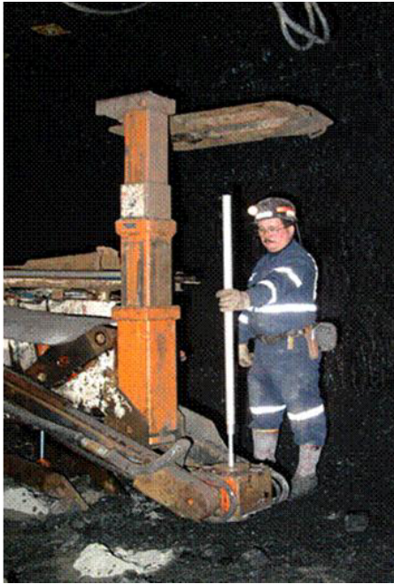
Figure 8. J.H. Fletcher and Co. has been investigating and evaluating different resin inserters, including a manual resin inserter.
