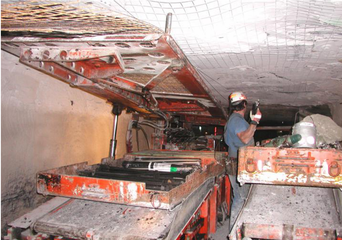
Figure 5. The J.H. Fletcher walk-thru bolting machine, with a material handling system (MHS), addresses material handling issues.
