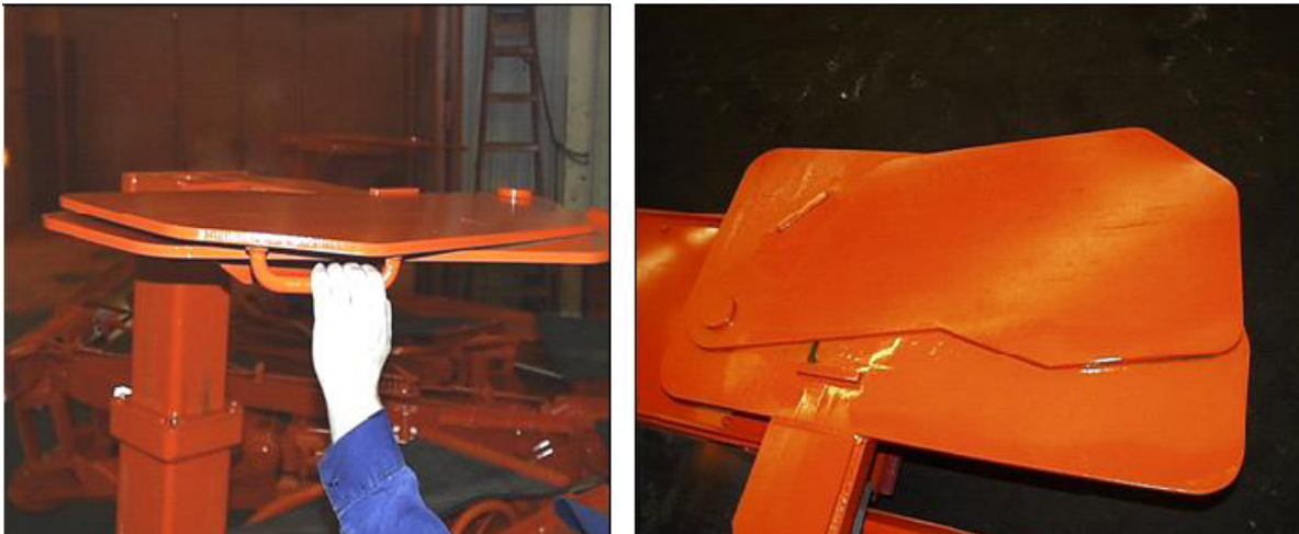
Figure 7. ATRS pull-out canopy extension pads provide additional protection to roof bolter operators.
