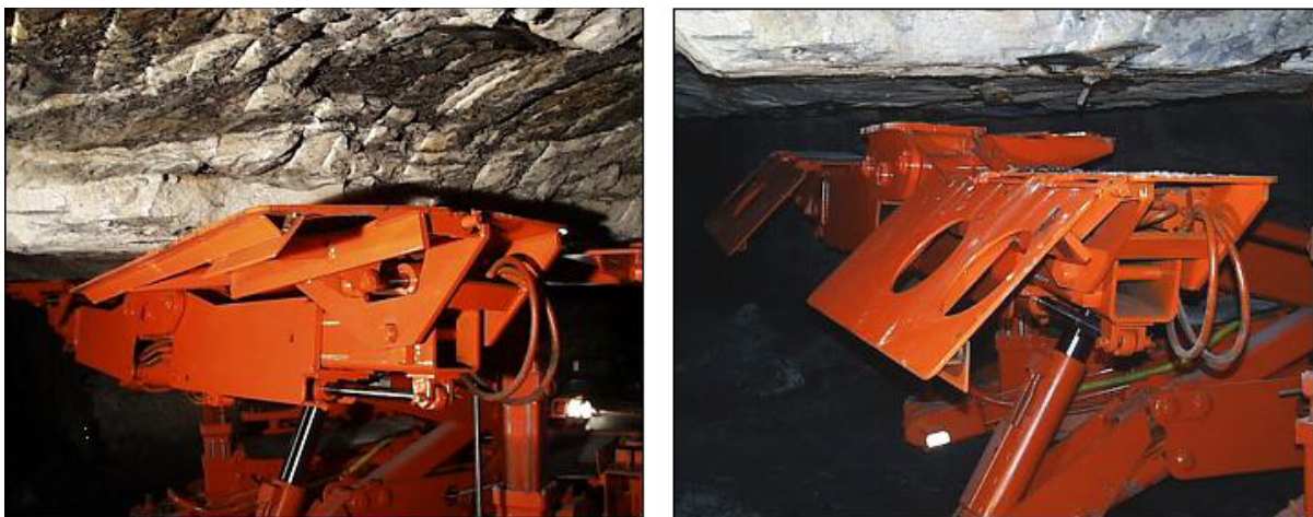
Figure 6. The ATRS deflector pad reduces the chance of a rock falling inby the ATRS and into the operator area.
