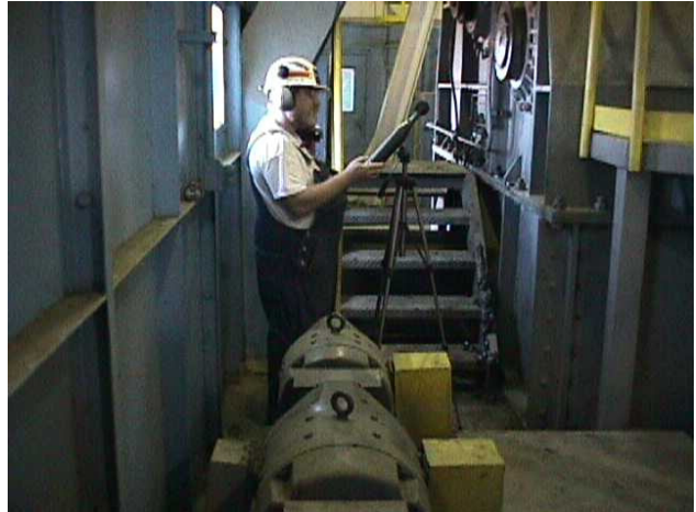
Figure 4. Example of noise measurement at a worker Location.
