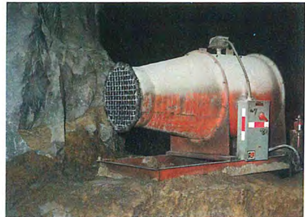
Figure 20. Axial vane auxiliary fan (note that the fan has a reducer that increases airflow momentum with a corresponding increase in entrainment and total airflow)
