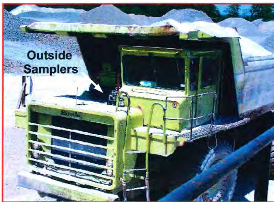
Figure 1 - Location of samplers on the front of truck.
