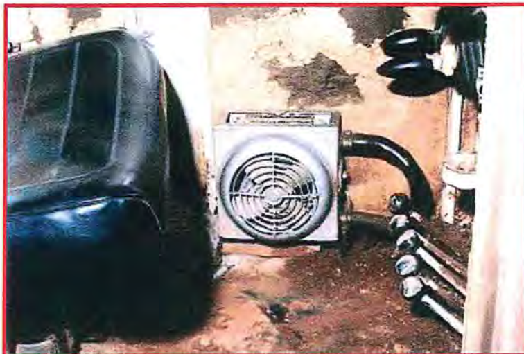
Figure 7 – Floor heater location inside enclosed cab.
