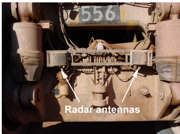
Figure 4. Preview radar system with two antennas.
