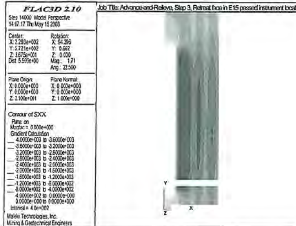
Figure 9. Horizontal stress contours (Sxx) at 17 ft into roof, Modeling step 3. (Lighter shades indicate stress concentration and darker shades indicate stress relief.)
