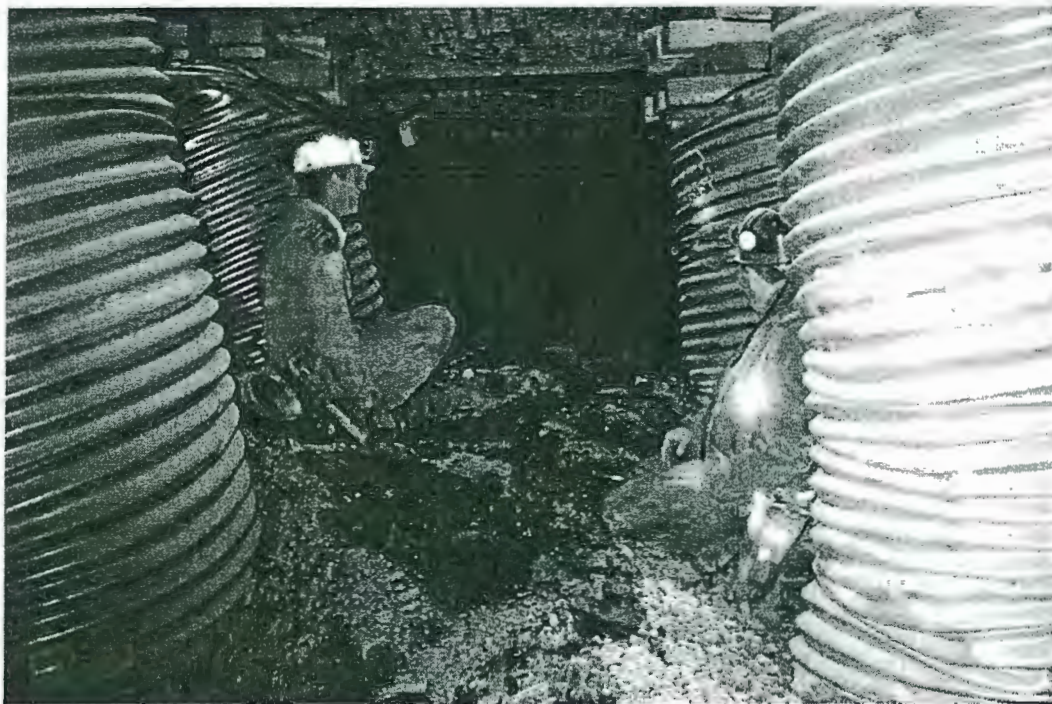
Figure 9. Large amounts of floor heaver shown outby the longwall face caused compression of the support which allowed it to develop sufficient load-carrying capacity for roof support in this installation.
