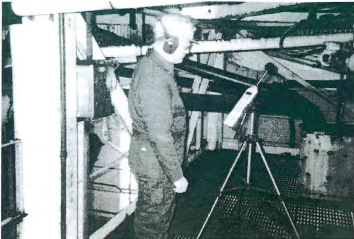
Figure 3: Noise measurement being made with a sound level meter.
