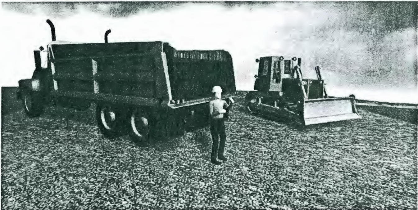
Figure 4: A computer actor recreates the fatal mistake made by a worker at a surface dump. The truck at left backed over the worker as he directed other traffic at the site.
