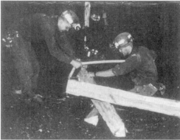
FIGURE 23.6 Timber support being set on a retreat mining section
