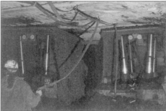
FIGURE 23.7 Mobile roof support (MRS) for retreat mining (photo by Chase 1992)
