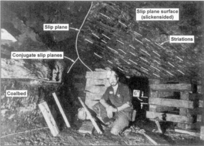
FIGURE 23.3 Fault in an underground coal mine (photo by G. Molinda)
