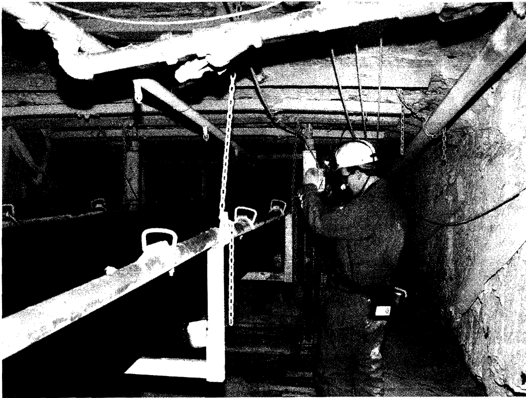
In a deep underground mine, water supplied from aboveground sources can result in pressures as high as 1,000 psig because of the water head. Photo by R. Conti, U.S. Bureau of Mines
