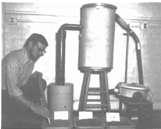
Figure 7.3. Demonstrating the separation of paper and fiber from plastic wire stripping waste with an air classifier.
