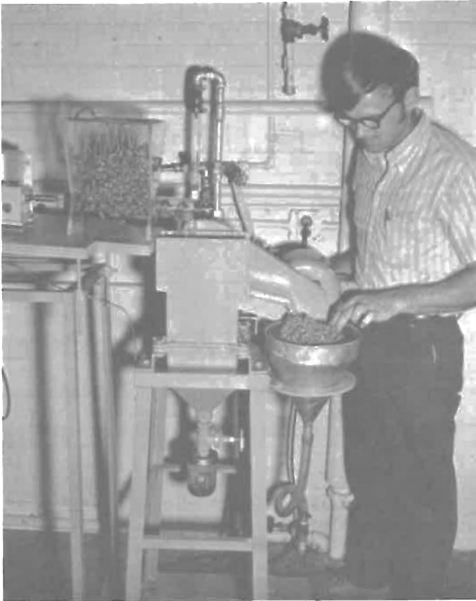
Figure 7.9. Laboratory jig, being used to concentrate wire from stripping wastes.
