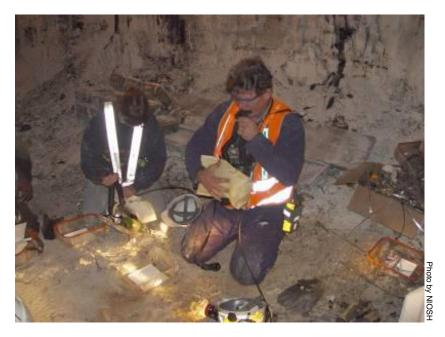
Figure 2. Miners preparing to escape by donning their self-contained self-rescuers (SCSRs).
