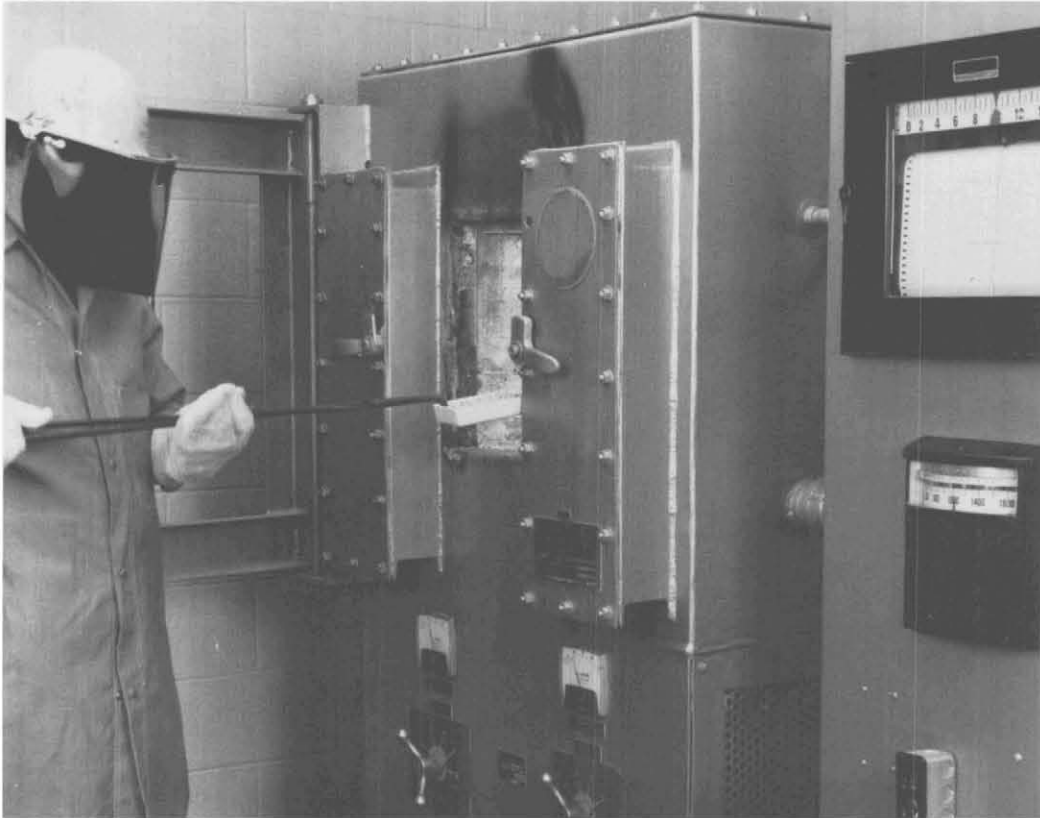
Figure 13.—Muffle furnace for limestone-gypsum roast tests.
