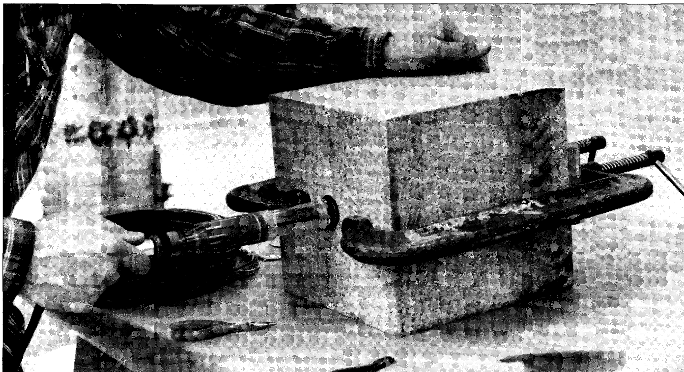
Figure 9. Installing the gauge for the glue-creep test
