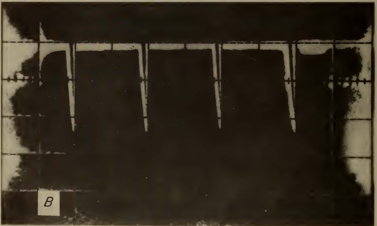
FIGURE 8B. - Switching regulator output waveform. Input voltage below nominal value.
