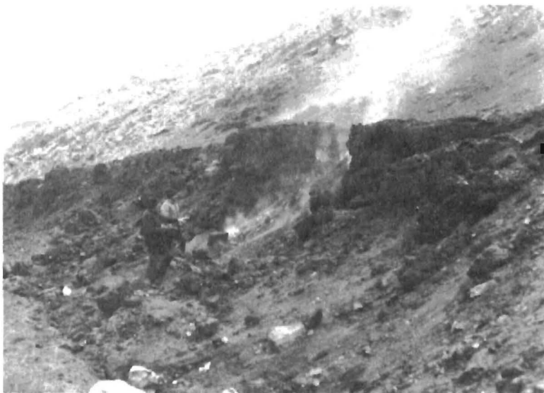
FIGURE 5. - A spontaneous combustion fire in a strip mine in Wyoming. The freshly uncovered seam is burning spontaneously.
