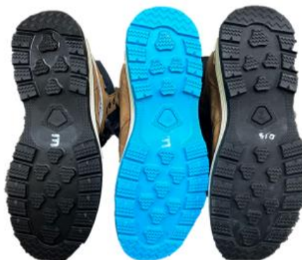
Figure 21: The A) STEPS slip tester used to collect experimental COF data between each shoe and floor and B) three of the eight shoes used showing the identical tread patterns.
