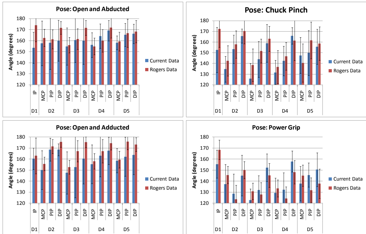
Figure 4: Comparison of Interphalangeal Joint Angles Between the Current and Previous (Rogers et. al., 2008) data sets. The data sets demonstrate similar trends between poses. Within a pose, the means between data sets vary up to 15°.
