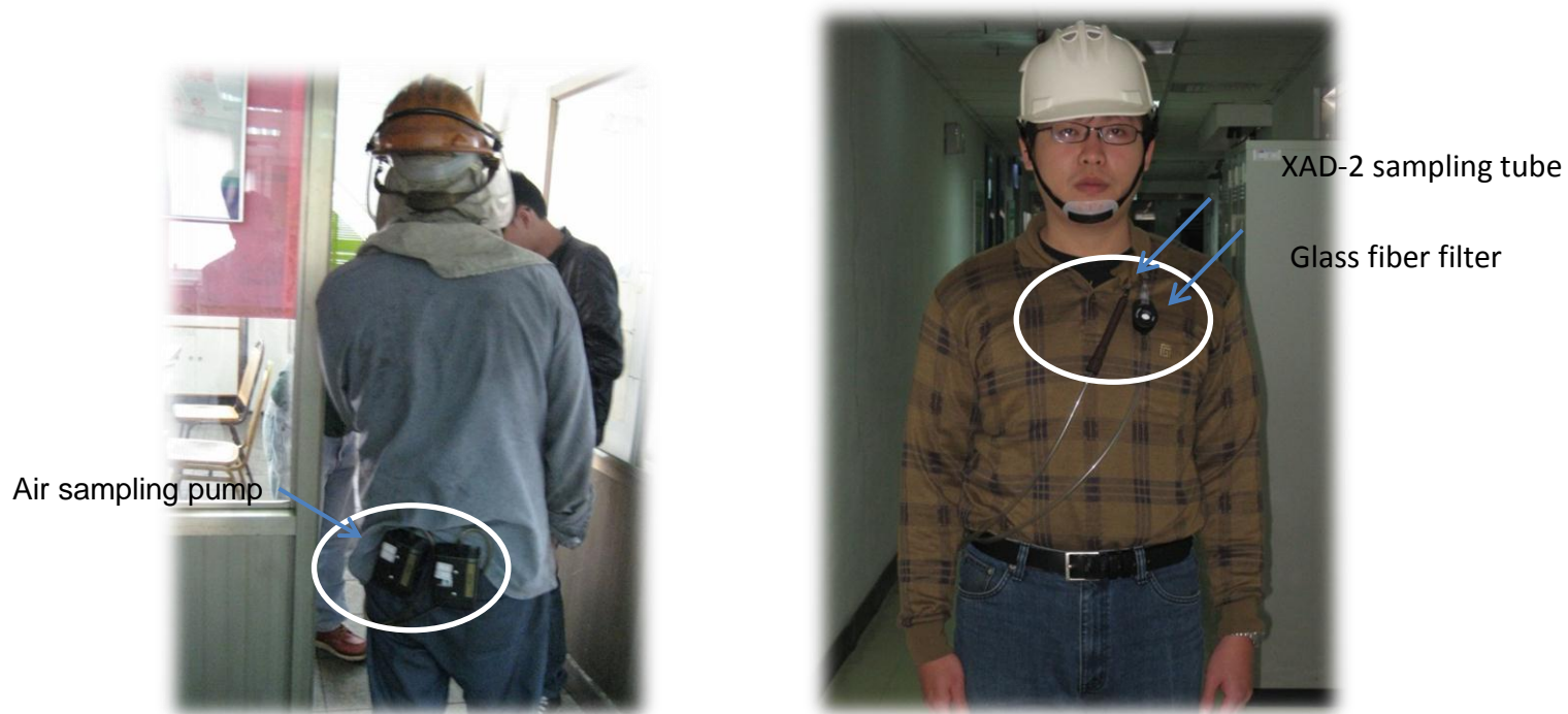
Figure 3. Personal breathing zone sampling. A) Each human subject carried two air sampling pumps attached onto their belts; B) A glass fiber filter cascade and a XAD-2 sampling tube for collecting particulate and vapor phases of PAHs, respectively, were attached onto the collar of the shirt.
