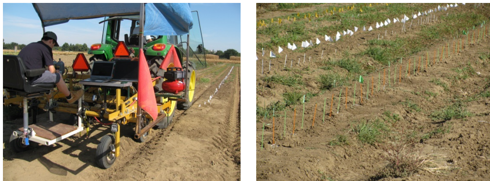
Figure 16. Field trials example. The worker controls watches the straws [plants) and adjusts the WBI as the knives open and close between straws.
