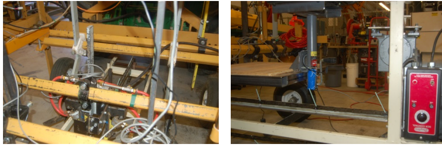
Figure 15. Controlled simulation of spaced-plants using a motorized continuous belt and colored plastic straws.
