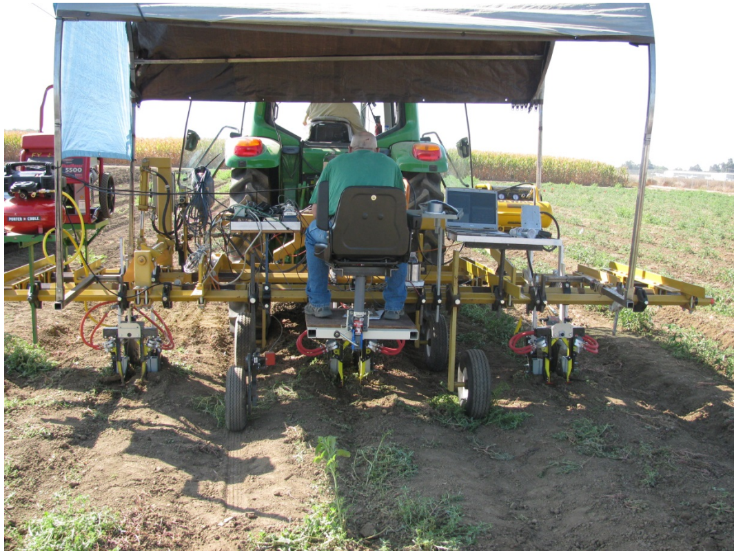
Figure 30. Three-row semi-automatic weeding system.
