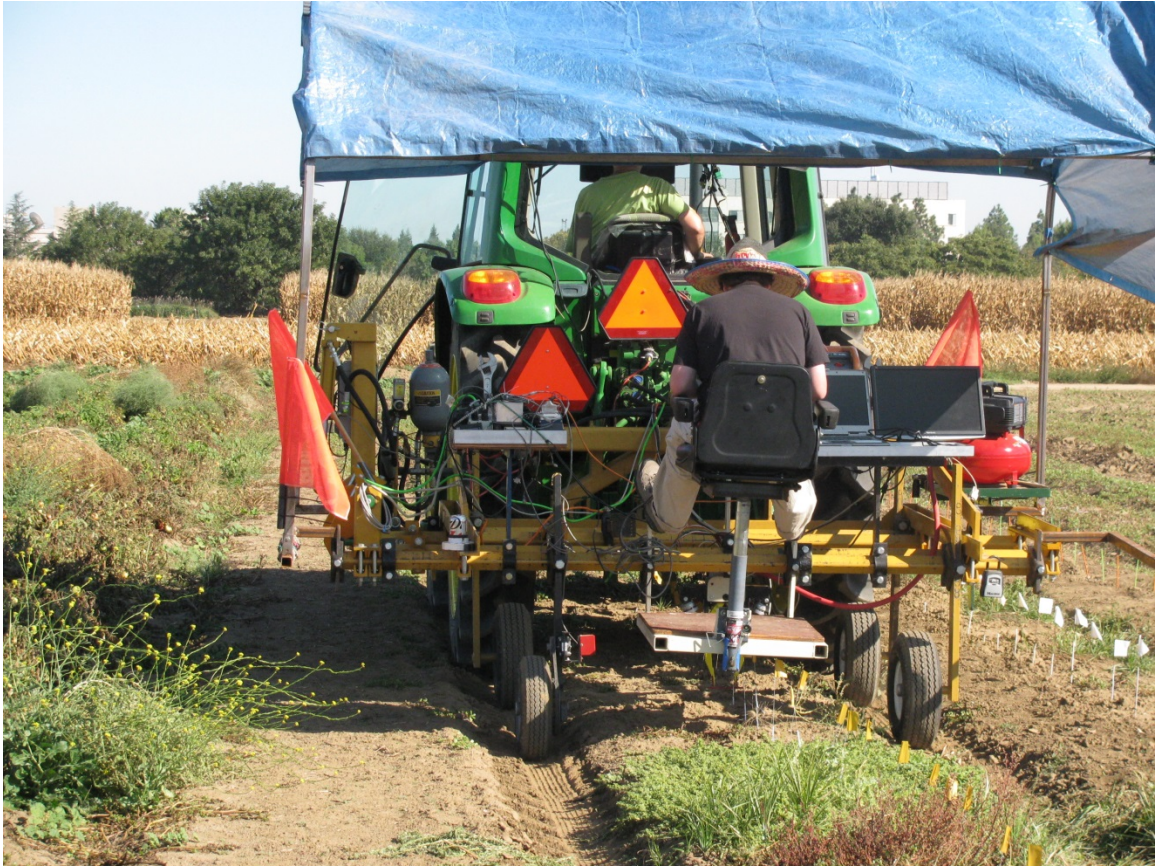
Figure 14. The controlled knives system and operator workstation implemented on an agricultural tractor.
