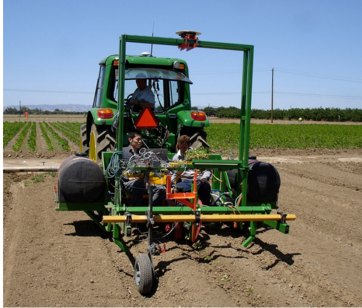
Figure 1. Photograph of the RTK-GPS automated transplant mapping system being used to plant tomato transplants on the UC Davis campus farm
