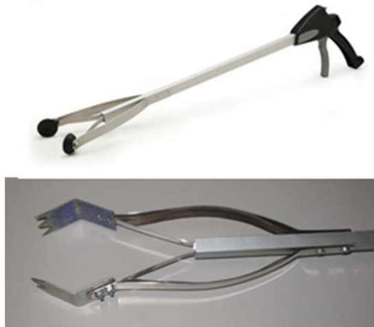
Figure 19. The E-Z Reacher [Top) and the modified weeding blades
