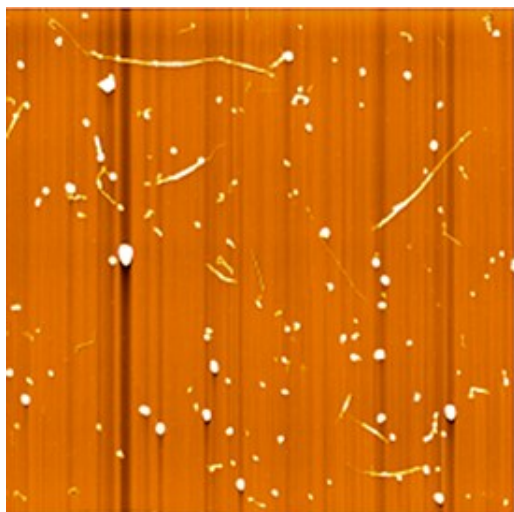
Figure 7. An AFM image of a 29 \mu g/ml CVD-SWCNT (HP grade, Helix, TX) sample deagglomerated by DMF with 5 minutes sonication [Scan size: 10 \mu m x 10 \mu m].
