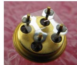
Figure 2: Packaged sensor element (uncapped).
