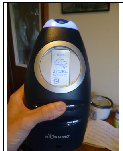
Fig. 1-2. NIOX Mino indicates when study subjects should inhale and exhale using an audio/visual display.
