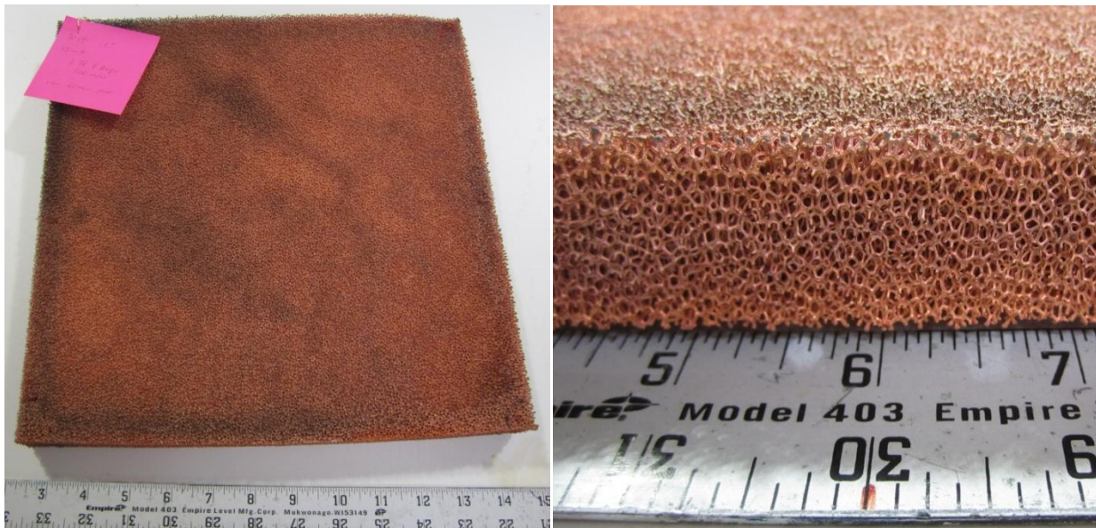
Figure 14. 12"x12" plated foam sample at 30ppi and 1" thick
