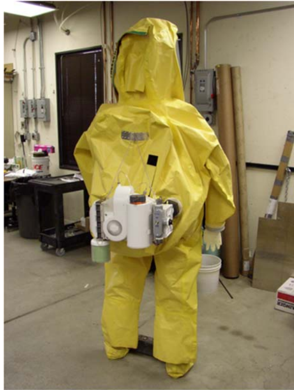
Figure 11. First generation prototype cooling system mounted onto manikin wearing a level-A Hazmat suit.
