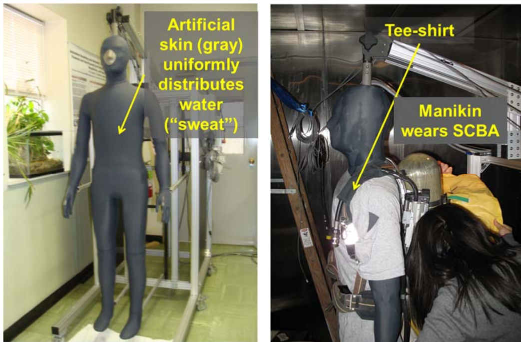
Figure 13. NIOSH thermal sweating manikin used to test first generation cooling system (left) and level A suit and cooling system being installed (right).
