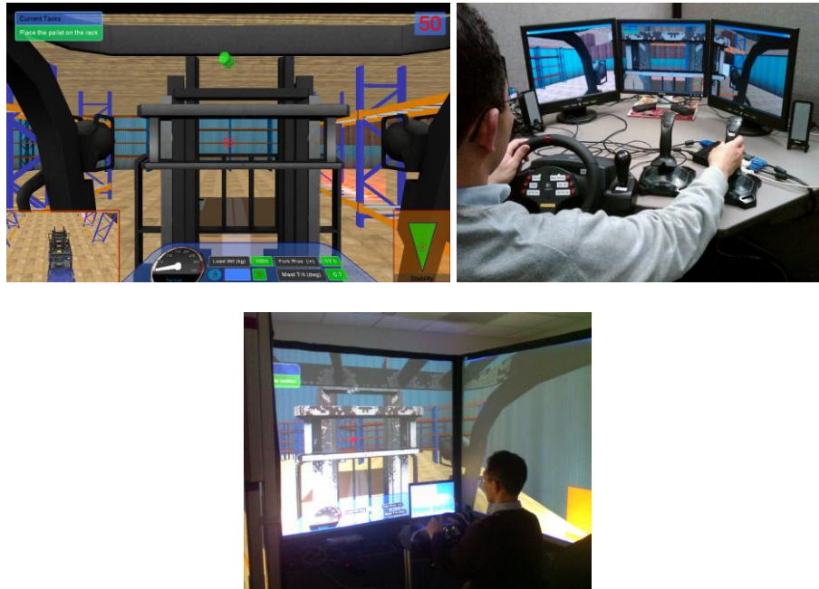
Figure 7. User interface of virtual forklift simulator: Truck dashboard (left), 3-monitor display (middle), and 3-projector immersive display
