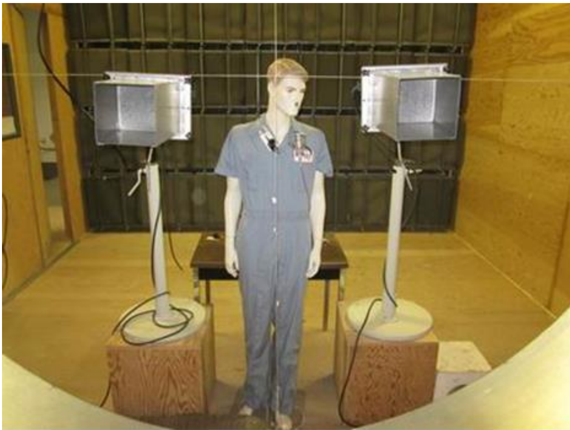
Figure 8. Photo of the test room of the LRR1 wind tunnel showing the full-size mannequin with the tested samplers and the two reference filter samplers.
