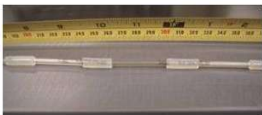
Figure 1. Test line consisting of 5-cm sections of test tubing connected together with 2-cm sections of silicon tubing.
