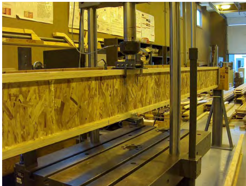
Figure 6. Static Testing of I-Joists Using Center Point Load
