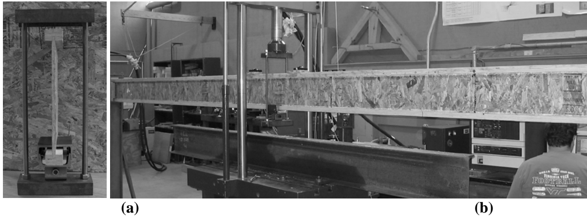
Figure 4: Static Loading of I-joists, (a) Loading Fixture, (b) I-joist Undergoing Buckling
