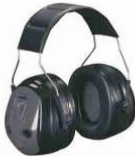
Figure 23. The Peltor Push-to-Listen (PTL™) amplitude sensitive circumaural, monaural earmuff, NRR = 26.
