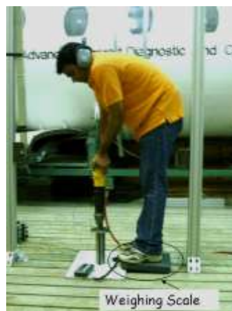
Figure 2.5: Human vibration tests.
