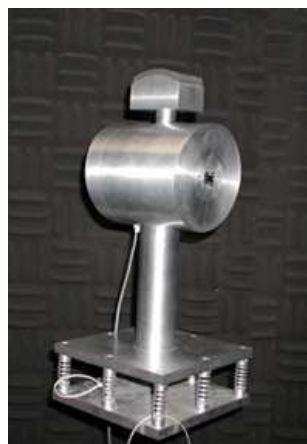
Figure 16. Acoustical test fixture (ATF) used to evaluate potential HPDs (electronic amplitude-sensitive, sound-transmission earmuffs) to support signal detection (protocol per ANSI S12.42—1995).
