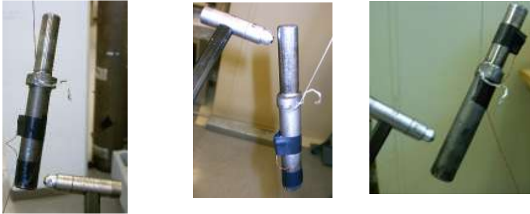
Figure2.23: Modal hammer testing a) tool center body, b) oval retainer and c) chisels.
