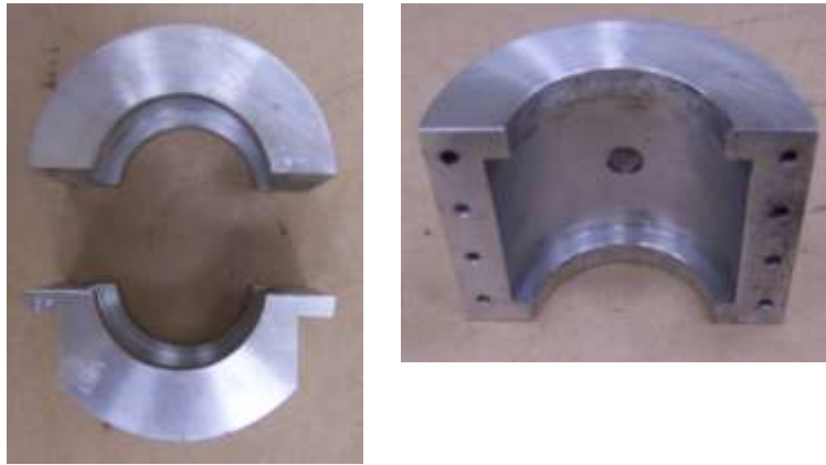
Figure 2.38: The aluminum encasement used to enclose the center body of the tool for the silencer experiments.
