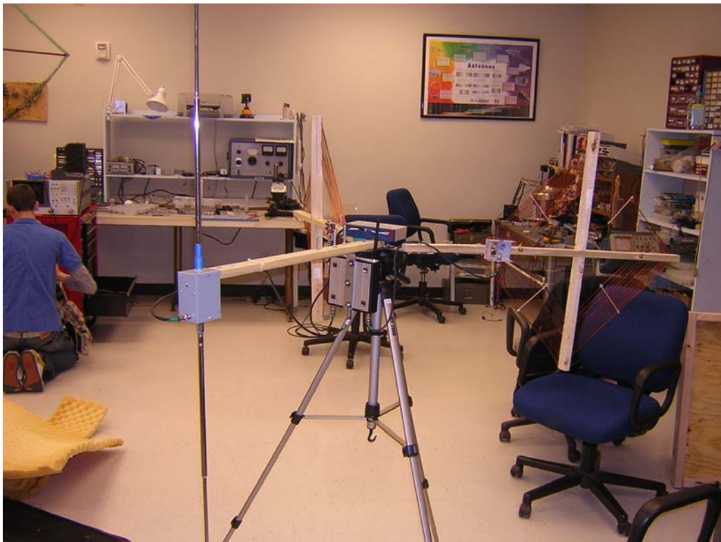
Figure 33: Q-Track receive antenna array: orthogonal magnetic antennas and vertical electric dipole.
