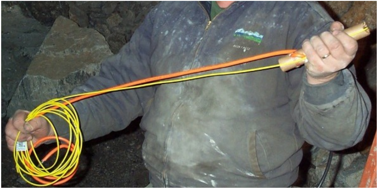
Fig. 9.5. A typical smoothwall blast primer showing 200 grain det-cord (thick orange) inserted into a stick of packaged emulsion explosive.
