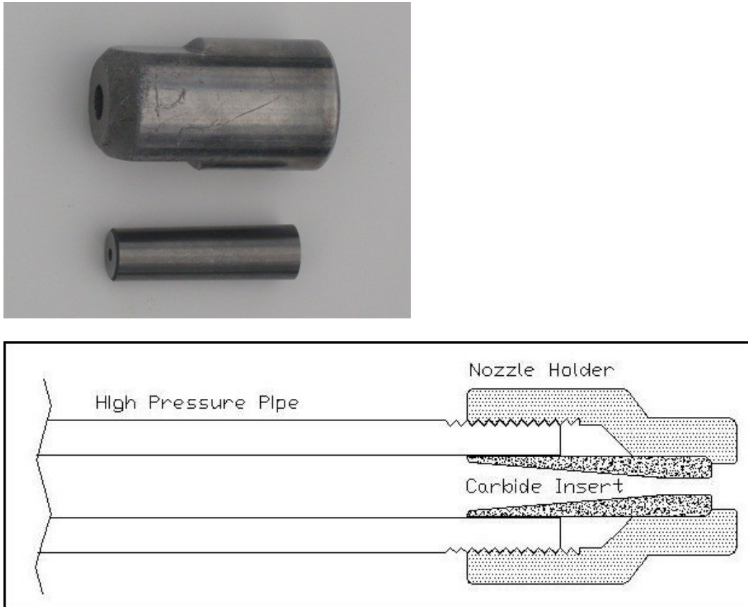
Fig 8.1. Single orifice continuous nozzle with holder.
