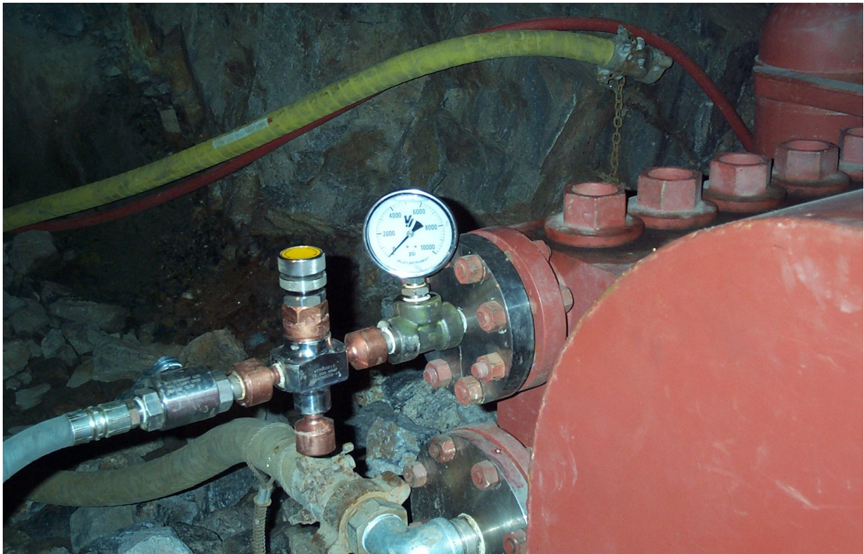
Fig 7.3. The pressure gage, flow control valve, and rupture disc assembly mounted on the Wheatly Quinteplex pump.
