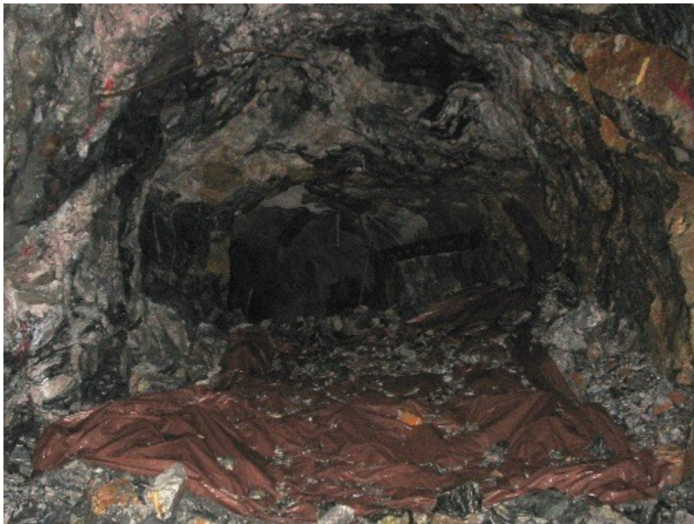
Fig. 10.31 Material removed in Experiment #6 waterjet test
