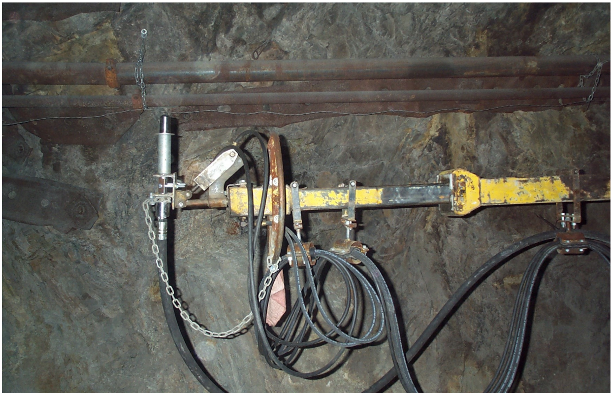
Fig. 7.7. The end of the hydraulic boom showing nozzle assembly mounting on the CSM waterjet scaling carrier vehicle.
