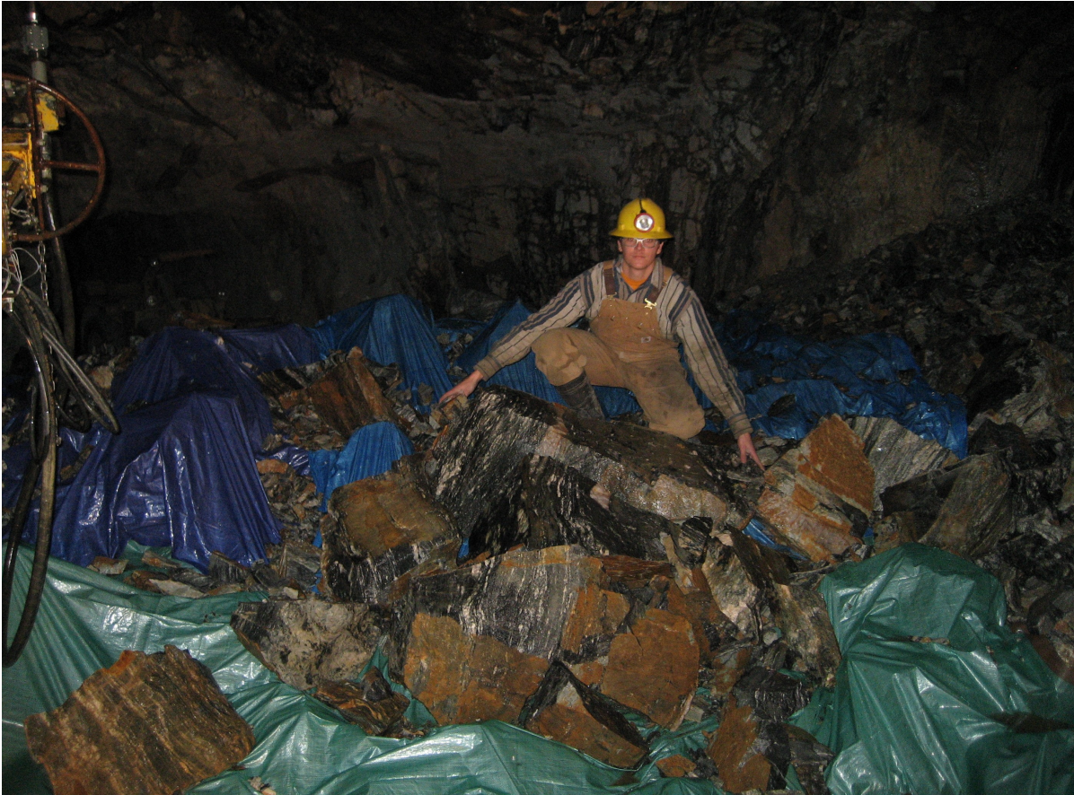
Fig. 11.4. The approximately four-ton slab scaled by the waterjet during experiment two.
