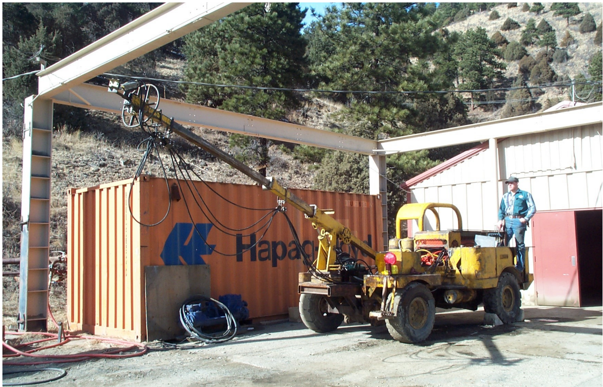
Fig. 7.6. The CSM waterjet scaling carrier vehicle.
