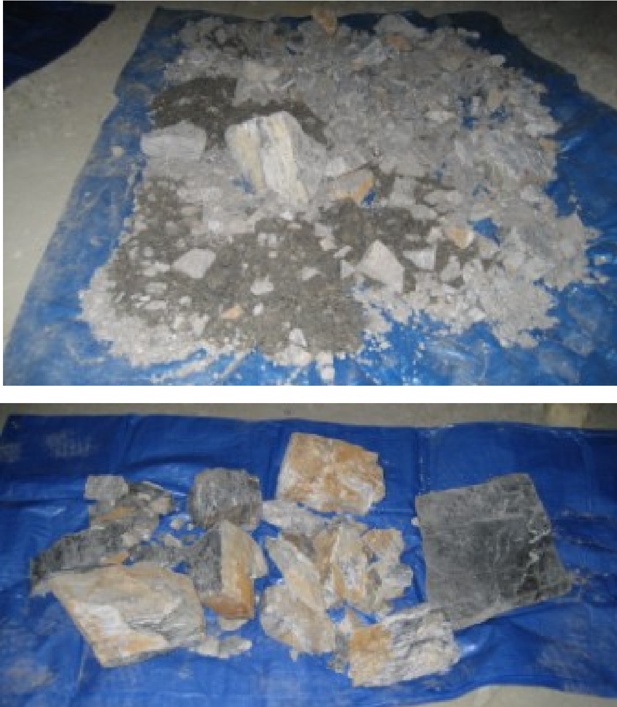
Fig. 11..9. Typical size distribution of material scaled by waterjet (upper) and a hand held scaling bar (lower).
