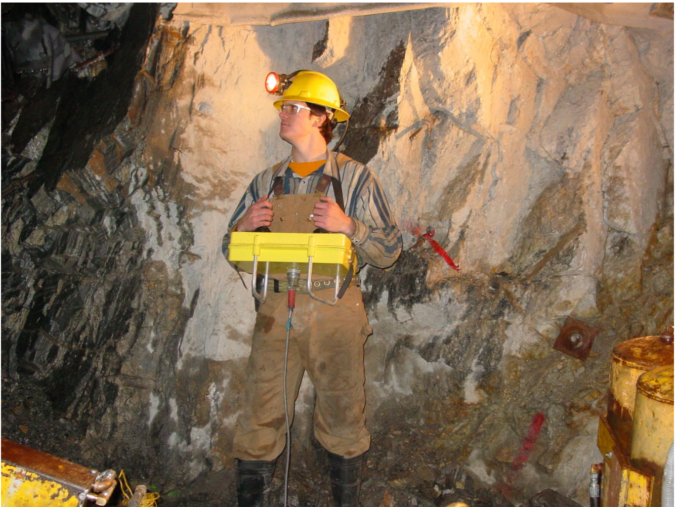
Fig. 7.8. The 12-volt electric joystick control box for controlling the motion of the hydraulic boom on the CSM waterjet scaling rig.
