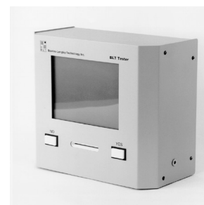
Photo 1, Original BLT tester as used in preliminary studies. Unit stores subject data on smartcards.
