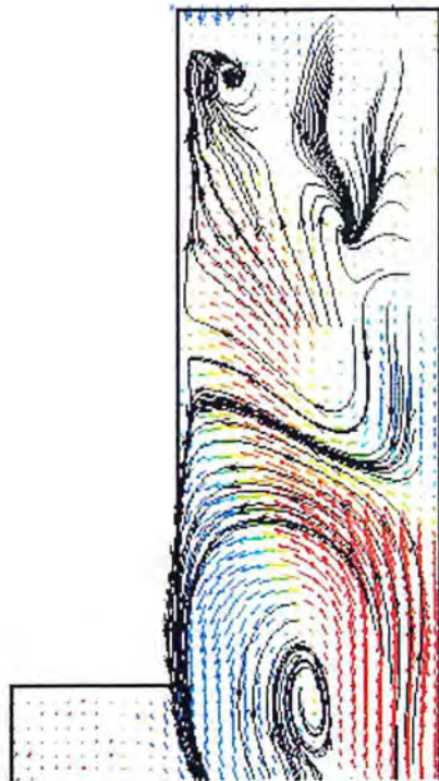
Figure 9a. Streamlines from PIV measurements with the machine mounted scrubber model for a 35 ft setback with a slab; Q_s/Q_{in}= 0.30 .
