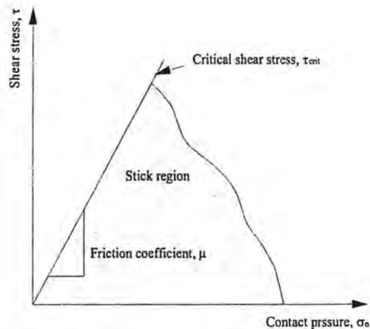
Figure 3-2 Linear Coulomb friction model
