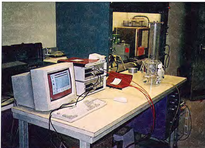
Figure 5. PSI metal monitor. Plexiglas sampling chamber is on right side of table.
