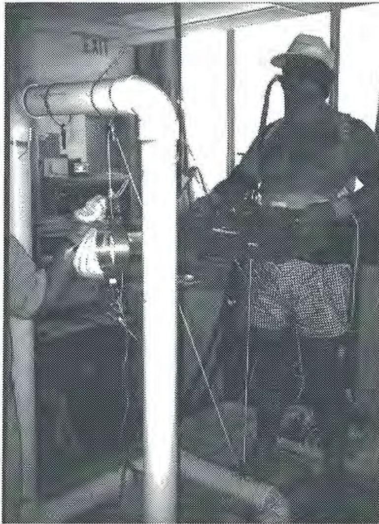
Figure 2.1. The experiemental apparatus for the second experiment. The blindfolded subject is about to receive the sagittally symmetric sudden load in a loose lifting belt trial without preload.
