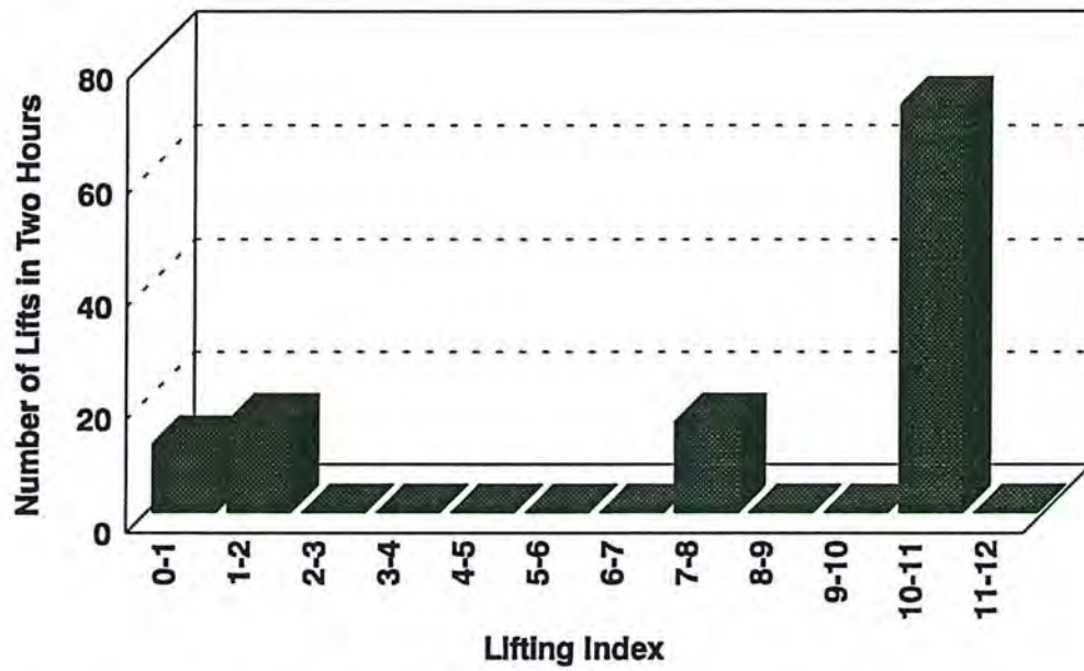
Figure 2. NIOSH Lifting Guide Assessment of a Mortar Mixer
