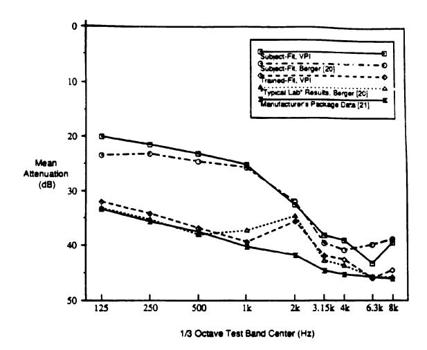
Figure 1. Foam earplug attenuation at each test frequency as fit by subjects using package instructions only (Subject-Fit, VPI) and by subjects receiving training from experimenter (Trained-Fit, VPI). Data collapsed across activity and measurement period. Berger (1988a) data and manufacturer's package data E-A-R (1989) shown for comparison.
