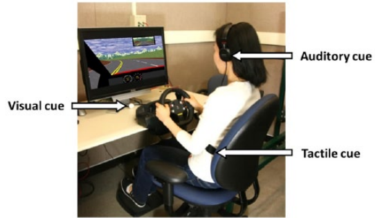
Figure 4. Experiment setup with multimodal stimulus and apparatus for Experiment 2 driving study.
