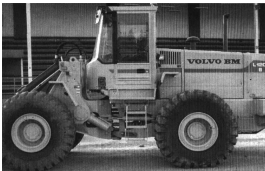
FIGURE 2. L120 B with the new Care Cab. It has a larger glass surface area and therefore confers better visibility. There is also considerably more room in the cab.
