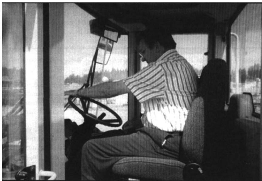
FIGURE 8. The steering-wheel setting in the new cab shows that the driver lifts his arm and shoulder a little higher and also loses a little contact with the backrest of the seat.
