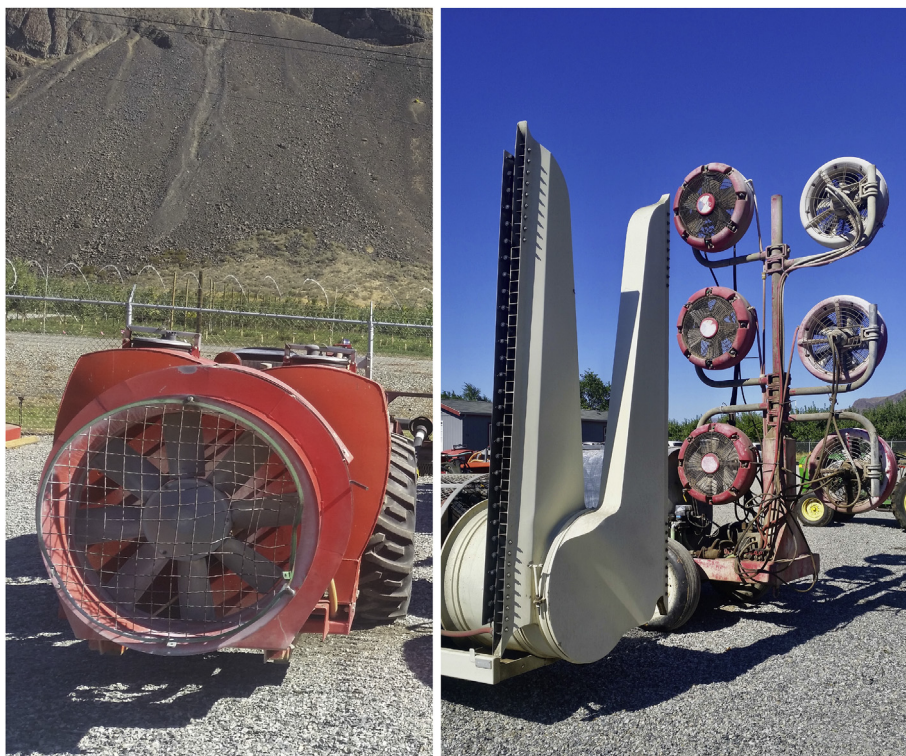
Fig. 1. From left to right: Axial fan airblast (AFA), directed air tower (DAT) and multi-headed fan tower (MFT) sprayer.
