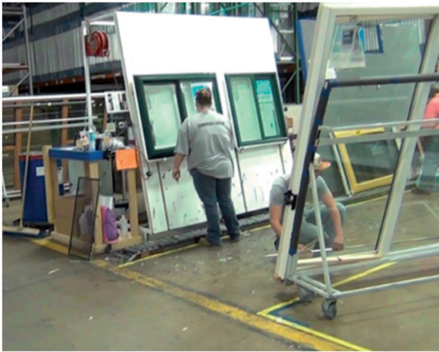
FIGURE 5. Adoption of the canted window orientation for the paint line allowing both standing and kneeling postures that reduce reaching.
