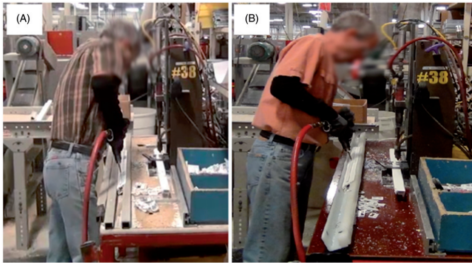
FIGURE 2. Worker performing fastening task on: (A) original workstation and (B) adjustable workstation.
