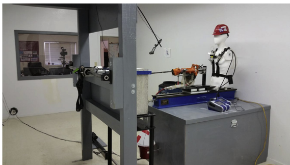
Fig. 1. The pneumatic drill mounted in the test bench system with rubber grips securing the handle and a Y mount supporting the drill near the bit. The drill mounting system slides on a lathe bed. After each hole is drilled actuators move the concrete block to a new location.
