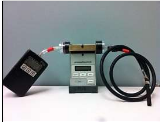
Figure 2. Sampling set up with pDR and SKC Aircheck Pump
