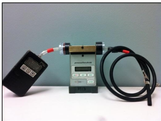
Figure 3.2. Particulate sampling train used for total particulate exposure measurements for shipyard observations. From down-stream to upstream: personal air sampling pump, pDR particulate monitor, 3.5 feet of conductive tubing, open sampling end attached in breathing zone of observed worker.
