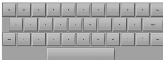
Figure 1. The four virtual keyboards evaluated. The keys were square and had a height and width of 13, 16, 19, and 22 mm. Across all keyboards, the spacing/gutters between keys was fixed at 2 mm. The printed letters on the keys are the same size across all keyboards.
