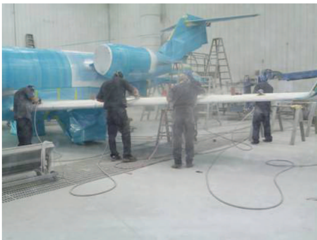
FIGURE 2. Employees wearing coveralls with a hood, goggles, gloves, and a full facepiece air purifying respirators while sanding an airplane inside a painting bay with pneumatic sanders that do not have dust control.
