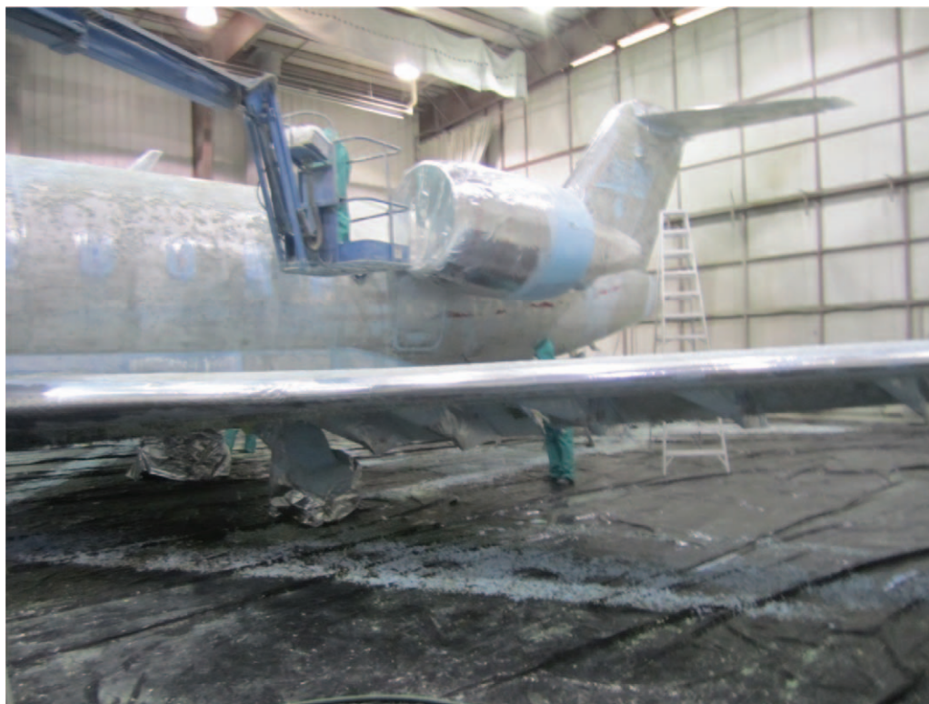
FIGURE 1. Liquid paint stripper applied to an airplane inside the stripping bay.
